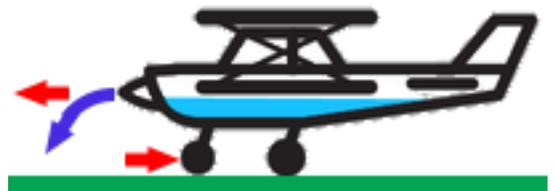
This is why jamming the throttle from idle to full has minimal effect on causing the plane to swerve. Things like engine torque and P-factor forces are mitigated by the nose wheel being continually pushed into the ground as the plane gains speed. This is also why the nose wheel is far more effective than the rudder when it comes to steering. (Now you know at least one reason why trainers typically have tricycle gear.)
