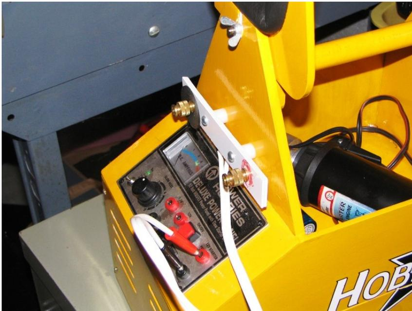
The standoffs allow me to wrap the wire shown in the picture for storage. I took care to mark the terminals black and red in order to keep the polarities straight. I clip the alligator clips from the chargers to the knurled knobs.
