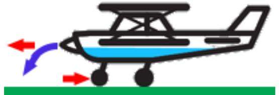
This is why jamming the throttle from idle to full has minimal effect on causing the plane to swerve. Things like engine torque and P-factor forces are mitigated by the nose wheel being continually pushed into the ground as the plane gains speed. This is also why the nose wheel is far more effective than the rudder when it comes to steering. (Now you know at least one reason why trainers typically have tricycle gear.)
